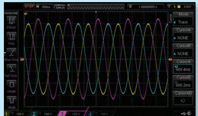
Three Phase Unbalance Voltage Test Captured
