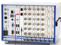
DEWE2-M7s with option DW2-LINK-PCIE-1-S
