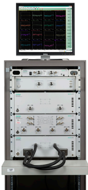
Rack mounted ShockLine VNAs
