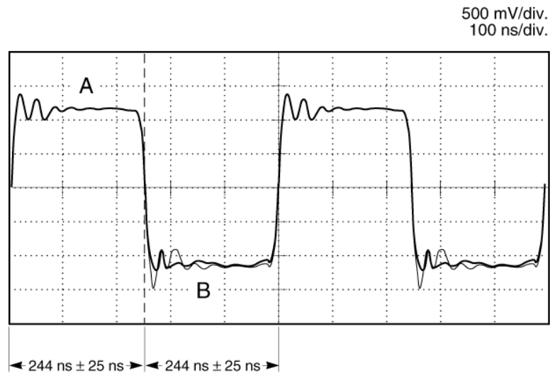
Figure 2-9. 2048 kHz Pulse Width Test
