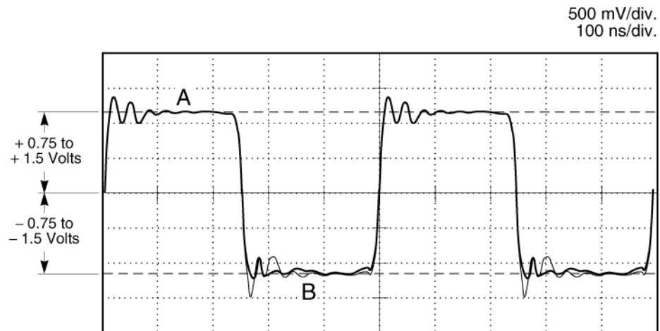
Figure 2-8. 2048 kHz Volt Peak Test
