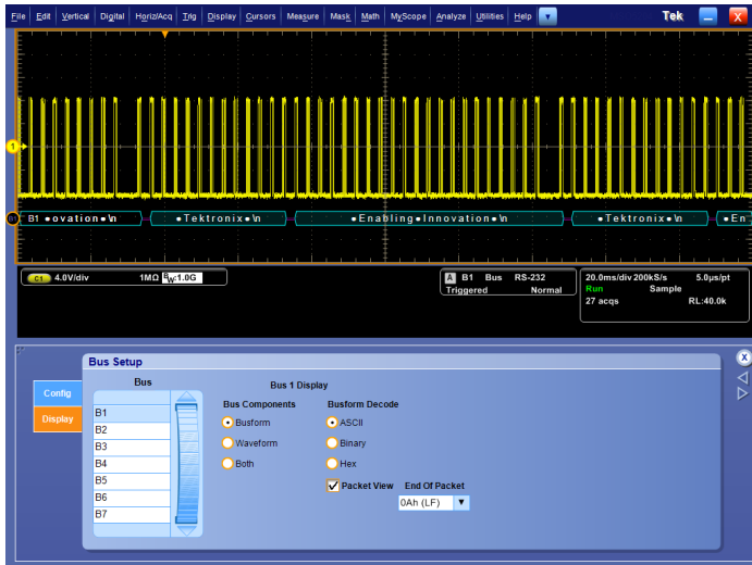
Packet View display of decoded RS-232 messages.
