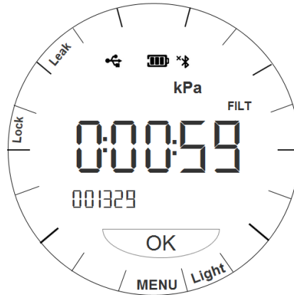
Figure 6 Pressure leak test setting interface
