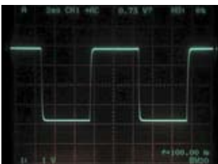
Input: 100 Hz square wave 300 Ap-p (Oscilloscope bandwidth 20 MHz)
