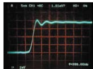
Input: 100 mA-p (Oscilloscope bandwidth 400 MHz)
