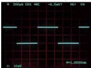
Input: 1 kHz square wave 200 mA-p (Oscilloscope bandwidth 400 MHz)
