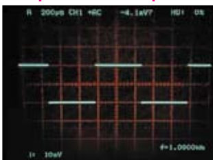
Input: 1 kHz square wave 200 mA-p (Oscilloscope bandwidth 400 MHz)
