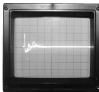
Fig 5-20 Fault located under the hot brush.
