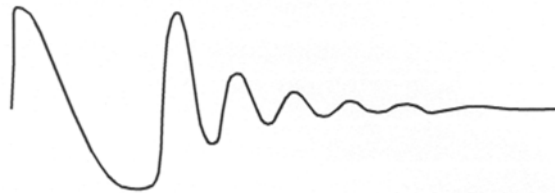
Fig 5.1: Example of a "ringing" wave pattern resulting from Surge Testing
