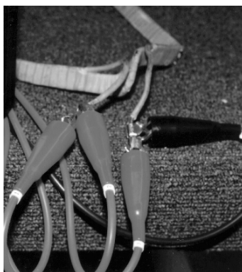
Fig 5-4: Example of how to connect the test leads for a surge test on a single coil or
