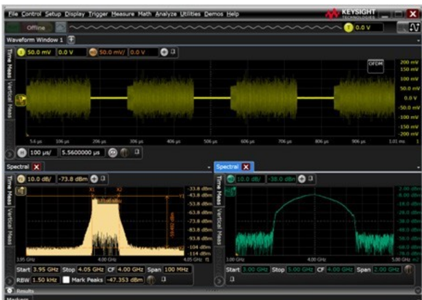
Use Infiniium capture and analysis of radar bursts, as shown in this OFDM example.
