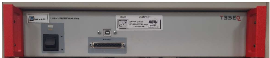
Figure 9 Detail of the 19" form factor CCN1000-3 upgraded to HFA-3-75 (notice the USB plug above the DB-37 connector in the front)
