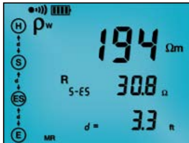
The Wenner test displays test lead connection, soil resistivity ( \rho ) test results, electrode spacing and resistance.
