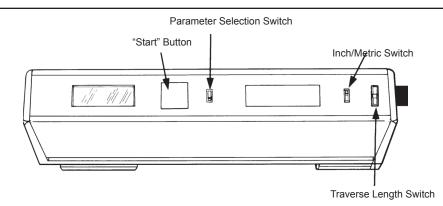
1. Set Inch/Metric Switch for inch (μin) or metric (μm).
