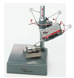
that the bracket with the Pocket Surf unit is tilted, using adjustment (2), to align with the tapered workpiece surface being measured.
