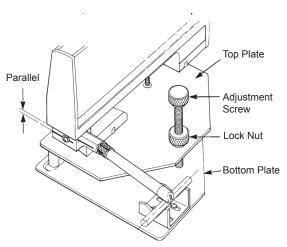
probe in its 90° position, to the fixture's Top Plate using the captive screw in the Top Plate.
