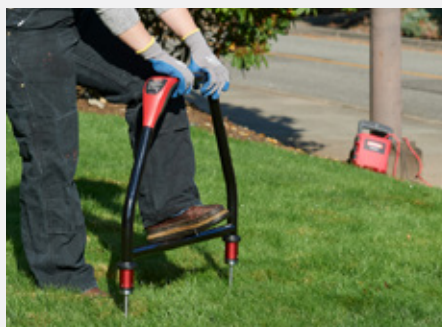
The AF-600 A-Frame pinpoints fault locations with the UAT-600-T Transmitter
