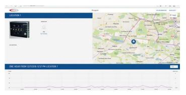
Vibration alerts are generated within seconds of them occurring and visualized and disseminated by Sentinel. The VMT can be set up with different alert trigger levels for different times of the day, and the reports contain sufficient detail for reporting and cause investigation.
