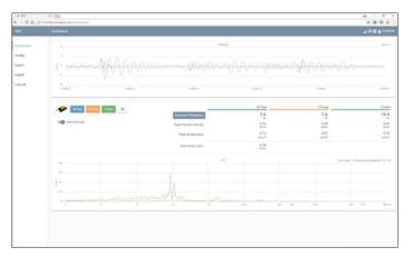
A variety of measurement parameters are available including velocity and acceleration in each axis, expressed as Peak, RMS and in SI (eg mm/s) or Imperial (eg in/s) units. The dominant frequency in Hz is calculated using either zero crossing frequencies or with FFT depending on the standard chosen. Realtime data can be viewed updated every second. A wide range of measurement weightings can be selected depending on the measurement standard chosen.
