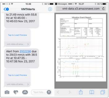
The vibration event may be set to trigger an SMS to a smart phone with an overview of the alert and a link to the alert report for viewing. The VMT can also automatically send the PDF report via email. The VMT can present the vibration data against a range of compliance curves.
