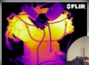
Heat buildup on cylinder heads of a compressor
