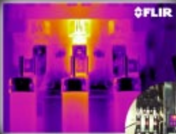
Connection problem on 200 Amp fused disconnect
