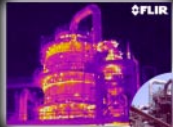
Thermal profile of a reactor refractory at a chemical facility
