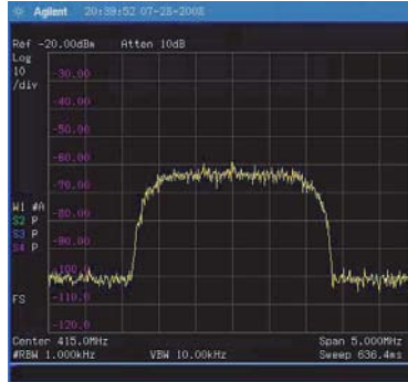
Scale indicator for quick vertical axis readout
