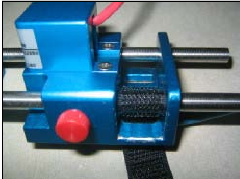
Figure 9: Installation on Small Diameter Pipes
