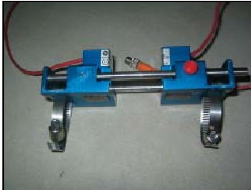
Figure 24: Metal Pipe Clamps Through the Inner Slots
