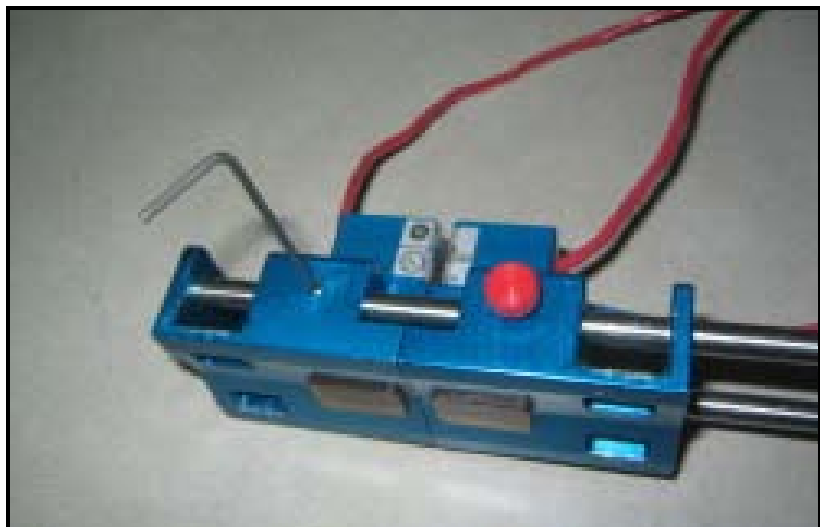
Figure 4: Loosening the Set Screws
