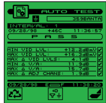
Auto Test results are time, date, and temperature stamped and can be stored, viewed, printed, or uploaded to StealthWare™ software.
