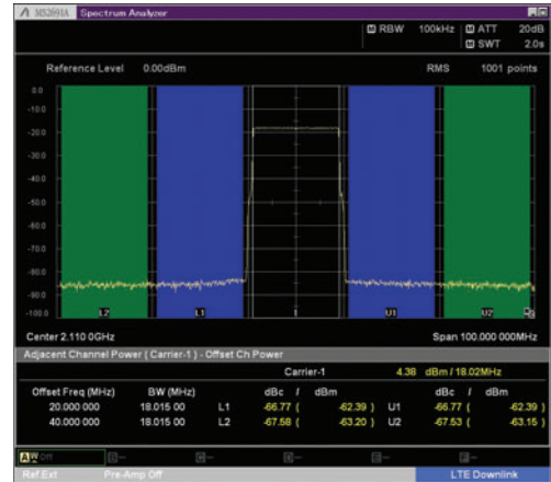
LTE FDD ACLR, 1 Carrier (E-TM1.1, Bandwidth 20 MHz)
