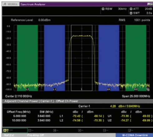
W-CDMA ACLR (1 Carrier) Waveform Pattern (TestModel1, 64DPCH)
