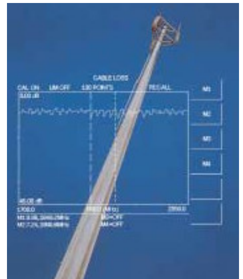
Verify cable insertion loss from ground level.
