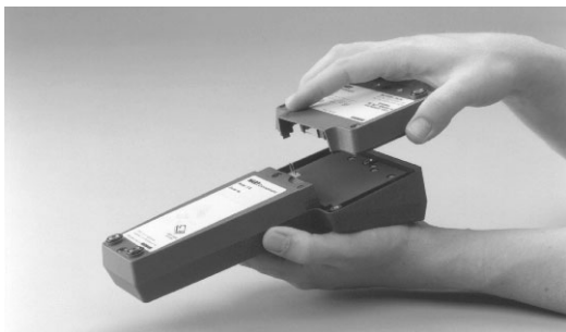
FIGURE 1-43. Battery Pack Removal.
