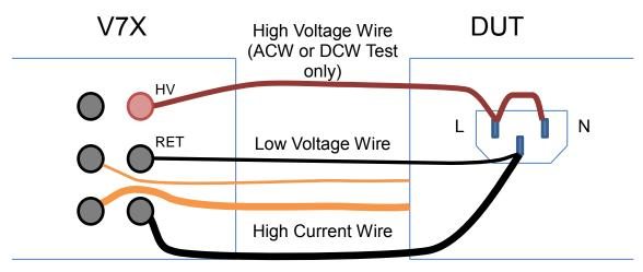
If the user needs to make optimum measurements of low impedances, particularly less than a few 10's of m $\Omega$ , then the following points should be considered -
