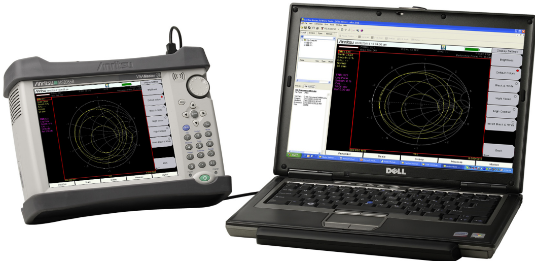
Figure 2-9. MS2035B Connected to PC via USB Mini-B
