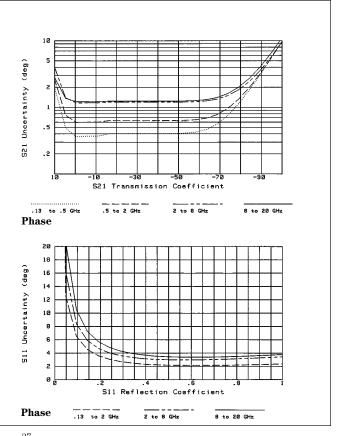
$^{37}$  The graphs shown for reflection measurement uncertainty apply to a one-port device.
