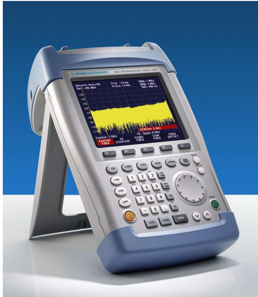
FIG 1 The Handheld Spectrum Analyzer R&S®FSH6 provides a frequency range of up to 6 GHz.
