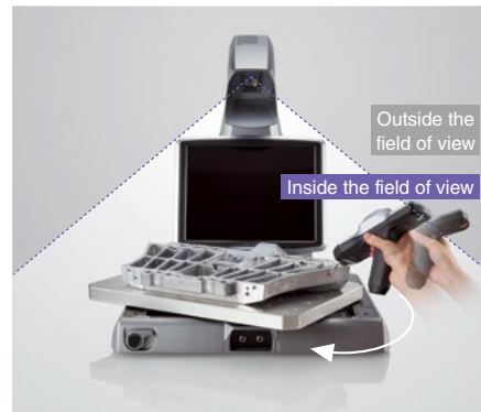
Rotate the stage to keep the probe within the field of view.
