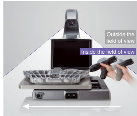
Move the stage to keep the probe within the field of view.
