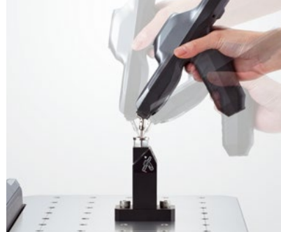
Easy calibration using the dedicated calibration jig
