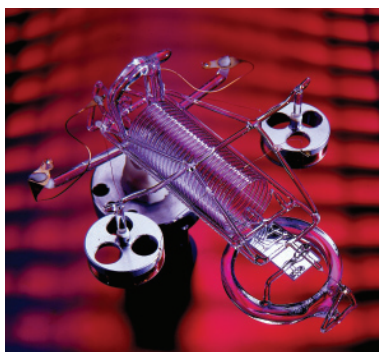
The 7250LP features a unique fused-quartz sensor. This rugged transducer offers unequalled precision and a stability of 0.0075% of reading per year. The media is in direct contact with the quartz, eliminating mechanical linkages and diaphragms, to provide the highest performance available in an automatic controller.
