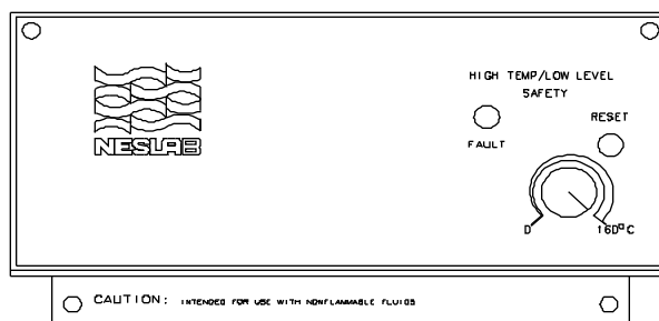
Pump Box (Front View)
