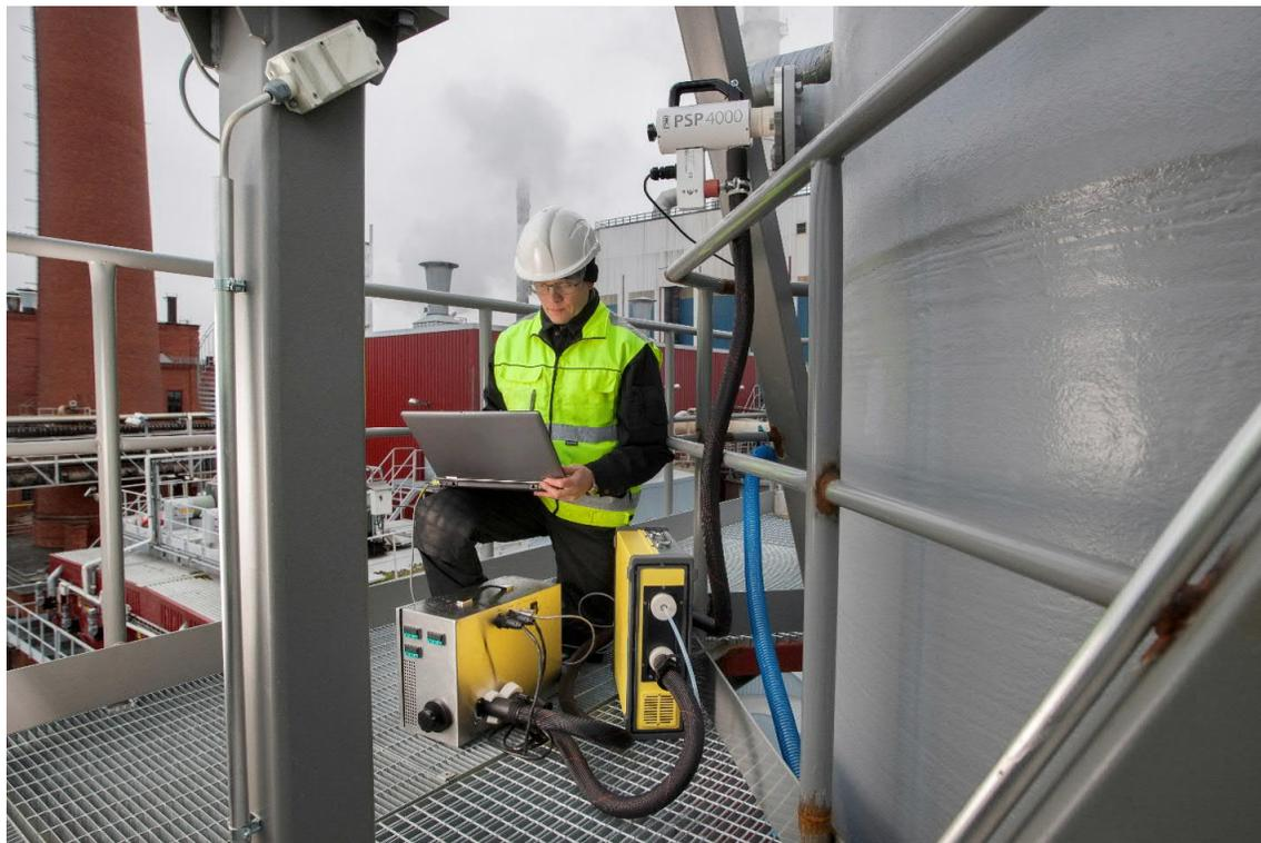
Gaset FTIR gas analyzers have been used for high-quality emission-related research already for more than a decade. Gaset analyzers have been used to measure pollutants and greenhouse gases from e.g. waste incinerators and wastewater treatment plants as well as for catalyst research.
