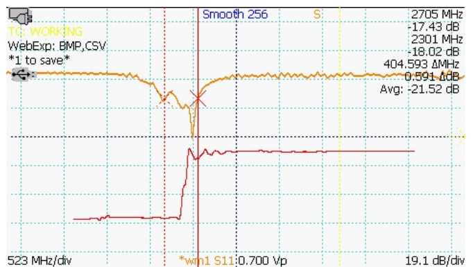
Figure 6: TDR and S11 return loss plots of a 2.4 GHz WiFi patch
