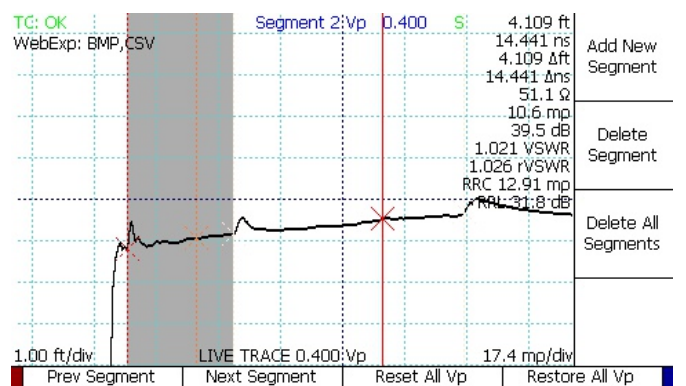
Figure 4: Multisegment cable with first segment VoP of 0.400.
