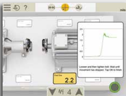
Soft Foot check on both machines.
