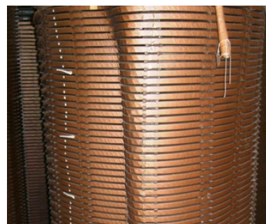
Buckling of winding
