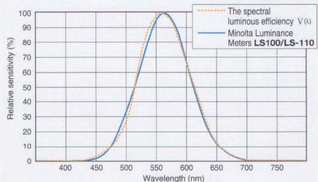
Ideally, the relative spectral responsivity of the luminance meter should match  $V(\lambda)$  of the human eye for photopic vision. As shown in the graph above, the relative spectral responsivity of Minolta Luminance Meters **LS-100/LS-110** is within 8% ( $f1'$ ) of the CIE spectral luminous efficiency  $V(\lambda)$ .
