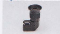
Angle Finder V<sub>N</sub> allows the measuring area and measurement display inside the viewfinder to be seen at an angle of 90° to the normal viewfinder optical axis. Angle Finder V<sub>N</sub> can also be focused and the magnification can be set to 1x or 2x.
