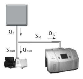
Figure 5 Parallel Operation
