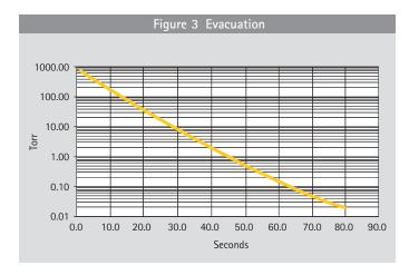
To reach the appropriate level in a timely fashion, it is necessary to select a pumping system based on the right pump characteristics, pumping speed and base pressure, as well as the right manifolds arrangement, conductance limitations and added volume considerations.
