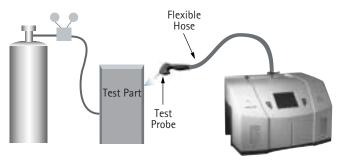
Figure 4 Locating Leaks - Inside Out
