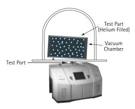
Figure 3 Measuring Leaks Inside-out
