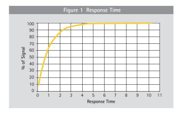
In order to quickly measure the signal in a vacuum application, the response time should be as short as possible. In general, a larger test volume will yield a slower response time. Also, a test volume connected to the detector by a long, narrow tube will negatively affect the response time, since helium must travel through the tube to the detector.
