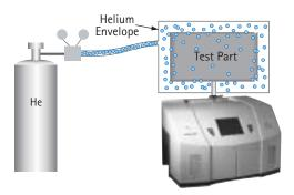
Figure 2 Measuring Leaks - Outside-In
