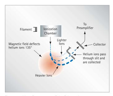
Figure 2 - Mass Spectrometer Tube Schematic
