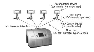
Figure 5 Accumulation - Inside-out
