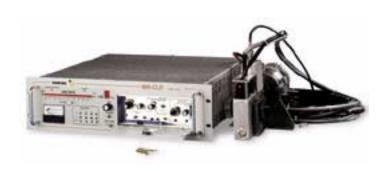
The Varian 990 CLD Component Leak Detector is a modular leak-testing package that can be integrated into virtually any testing system. The electronics module of the 990 can be separated from the sensing module and vacuum pumps by as much as 15-feet, permitting a high degree of flexibility in your system design.
