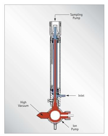
Figure 3 - Selective Ion Pump Detector
