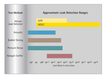
Figure 1 - Leak Test Methods Comparison
