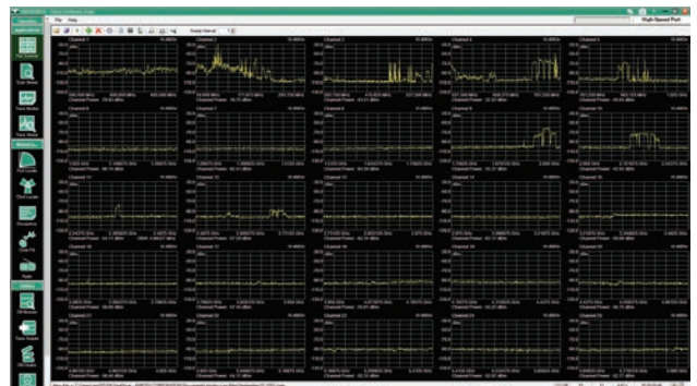
Use the High Speed Port Scanner Monitor Multiple RF Channels with a Single Site Master MS2089A on a Single PC Monitor
