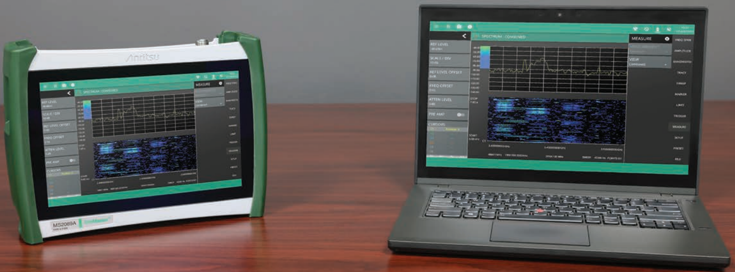
Laptop PC Running Remote GUI Application with Wi-Fi Connection to MS2085A/89A
