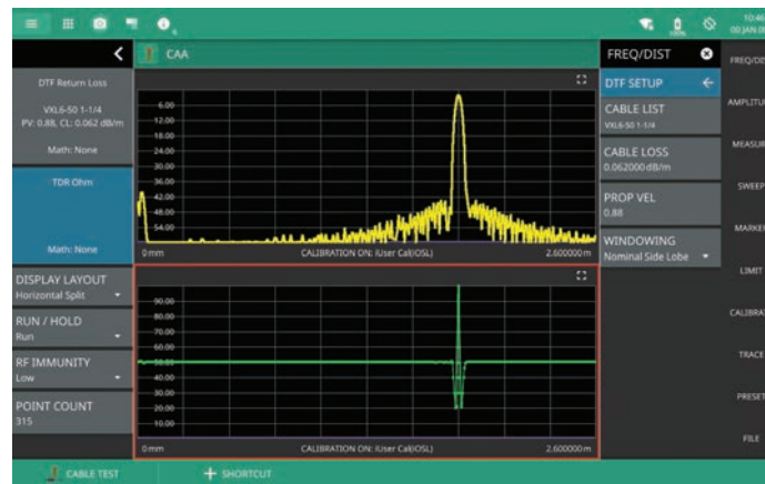
Split Screen Showing DTF and TDR Measurements
