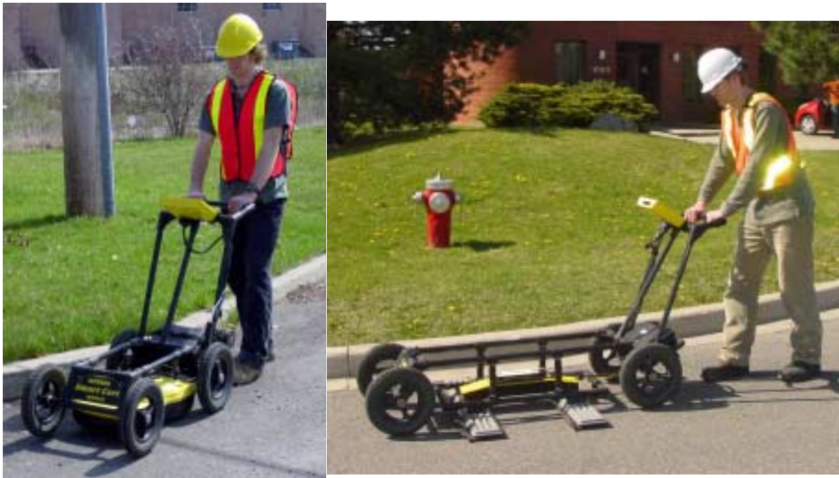
Figure: 4-2 Noggin 250 SmartCart (left) and Noggin 100 SmartCart (right) in operation.
