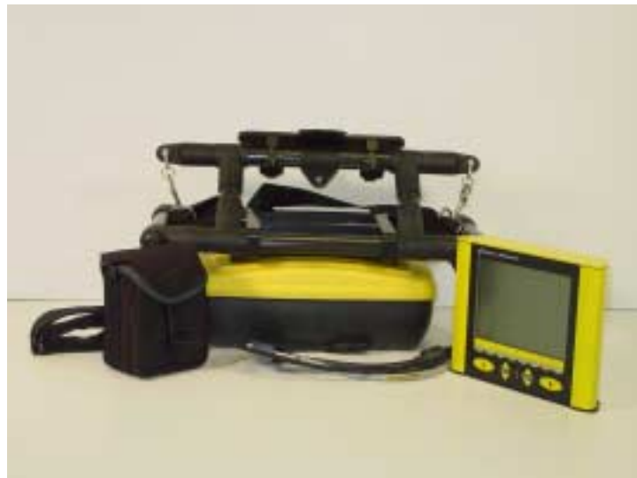
Figure: 7-3 The Rock Noggin system components after removal from the shipping case. From left to right are the belt battery, the Noggin already attached to the frame and the Digital Video Logger (DVL). The system comes partially assembled. To continue with assembly from this point, see Figure 7-11 and later.
