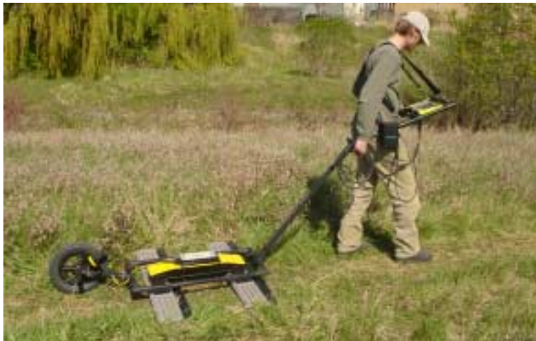
Figure: 5-2 Noggin 100 SmartTow configuration in use. Note the belt battery for power and DVL carrier for conveniently carrying the DVL in the field. The cable runs from the electronics housing and up the handle secured by velcro straps.
