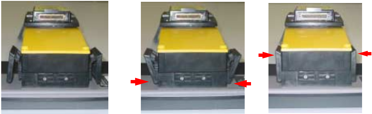
Figure: 3-3 Latching the electronics to the antenna.
