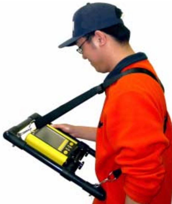
Figure: 9-2 The DVL and control module can be attached to the optional DVL Carrier for hands-free operation. The DVL can be adjusted to optimize the view angle.
