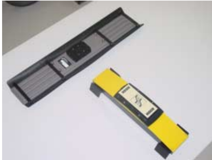
Figure: 3-1 Noggin 100 assembly of electronics to antenna.
