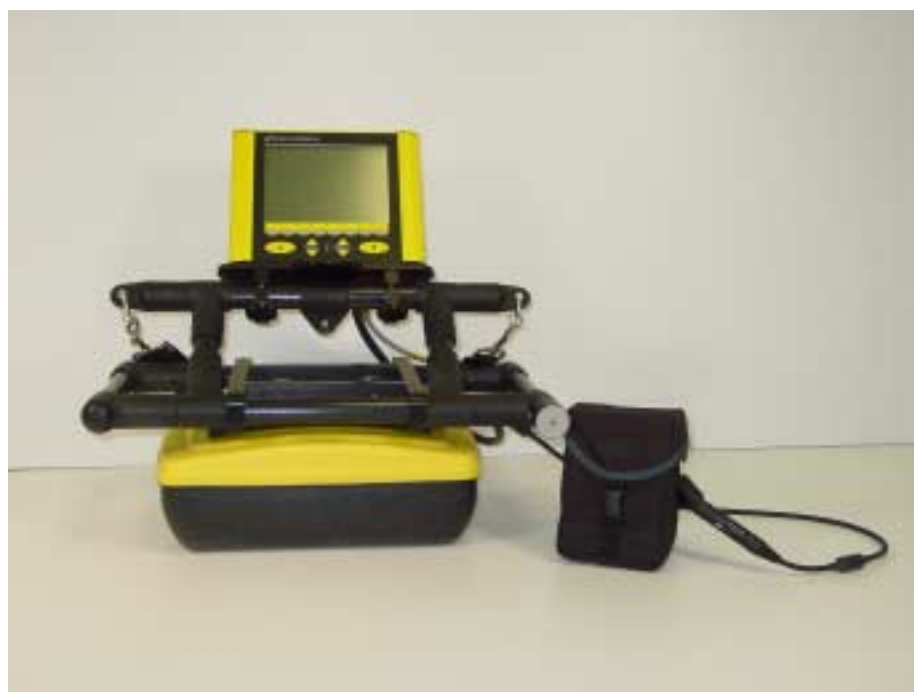
Figure: 7-15 The Rock Noggin system is now completely assembled and ready to be turned on.
