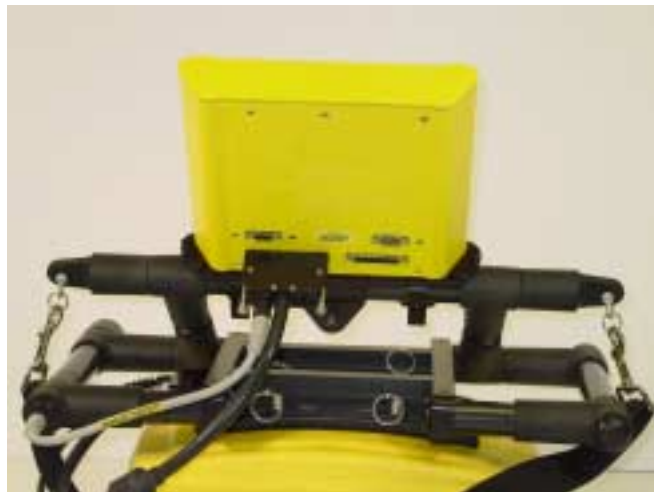
Figure: 7-13 Attach the end of the cable with the 37 socket (female) connection to the back of the Digital Video Logger (DVL). Use a slotted screwdriver to tighten the connection.
