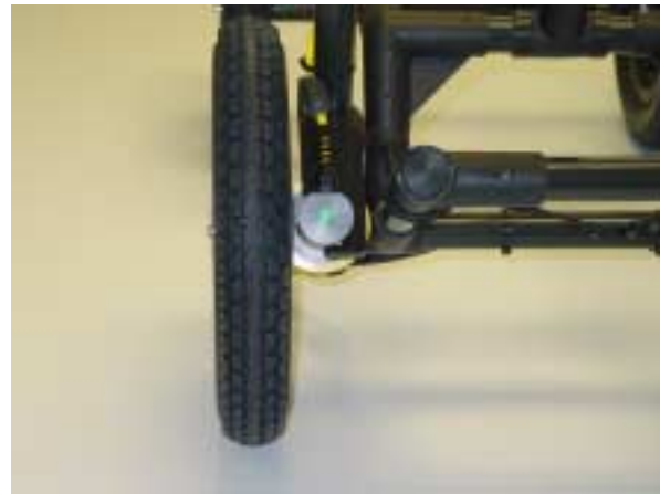
Figure: 4-6 If the odometer wheel does not make good contact with the wheel, use a hexagonal wrench to loosen the 2 screws (left) and pivot the odometer outward so when the wheel is attached the odometer rolls continuously (right).
