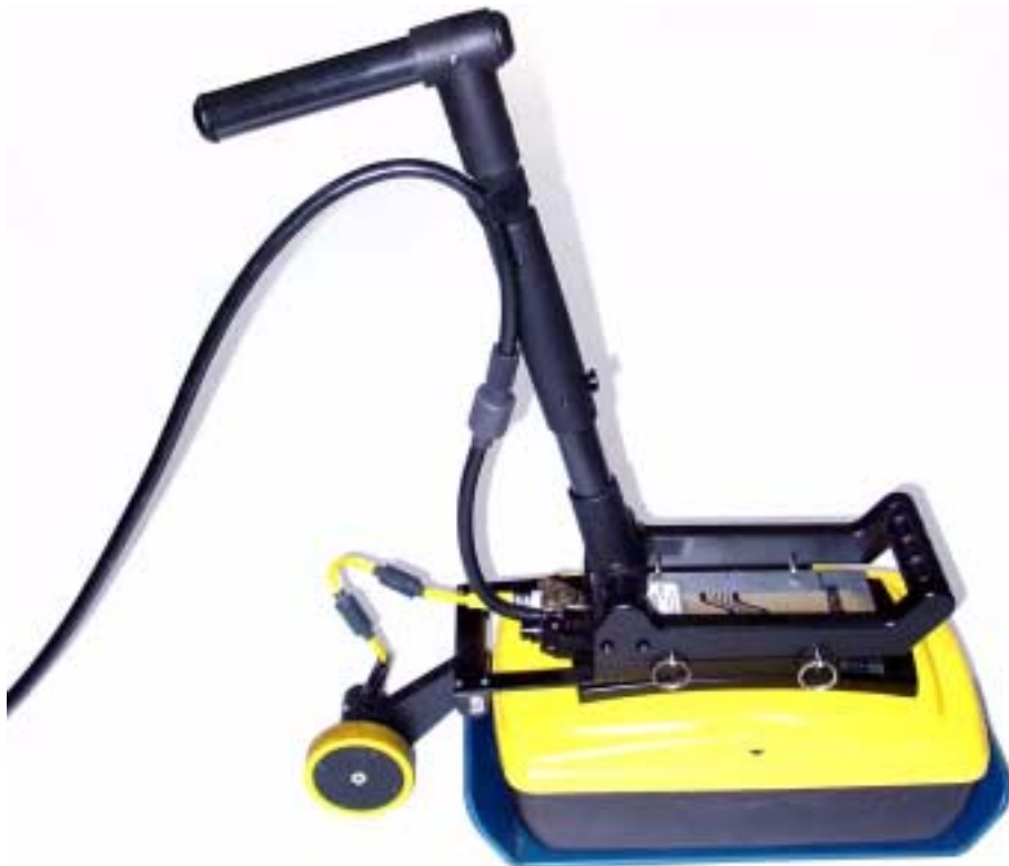
Figure: 6-6 The full-length SmartHandle is shown in Figure 6-1. The SmartHandle can be shortened by removing the center handle section using the thumb-screws. Use the Velcro straps to secure the cable onto the SmartHandle, ensuring there is excess cable near the connection at the Noggin to allow the SmartHandle to pivot up and down without straining the cable.
