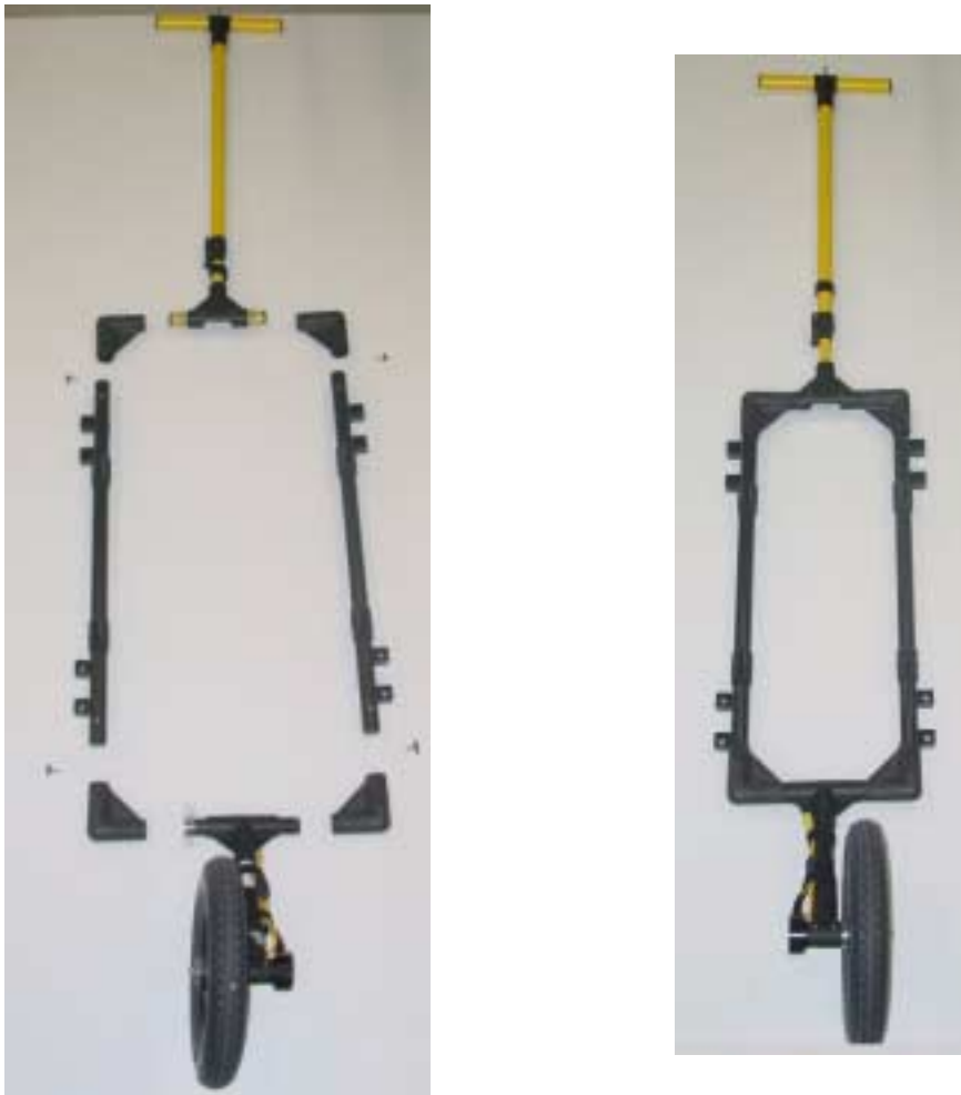
Figure: 5-3 The Noggin 100 SmartTow frame parts (left) and assembled (right). Ensure the antenna post blocks face outward before assembling. The pieces are connected using the 4 thumb screws as shown in the figure below. The Handle and Big Wheel odometer are not connected to the frame with thumb screws but held in place once the antennas are attached.
