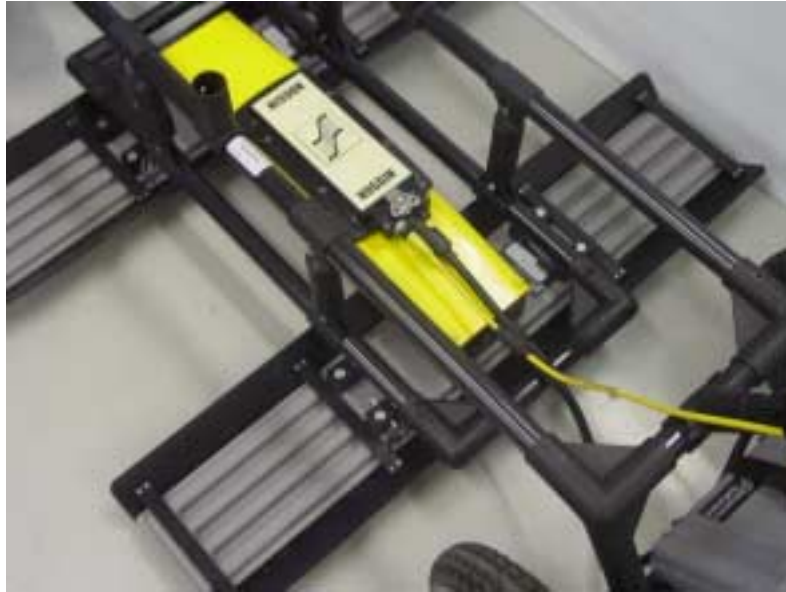
Figure: 4-13 Connecting the Noggin-to-DVL cable to the Noggin 100 electronics. After this connection is made, connect the yellow odometer cable to the round receptacle.
