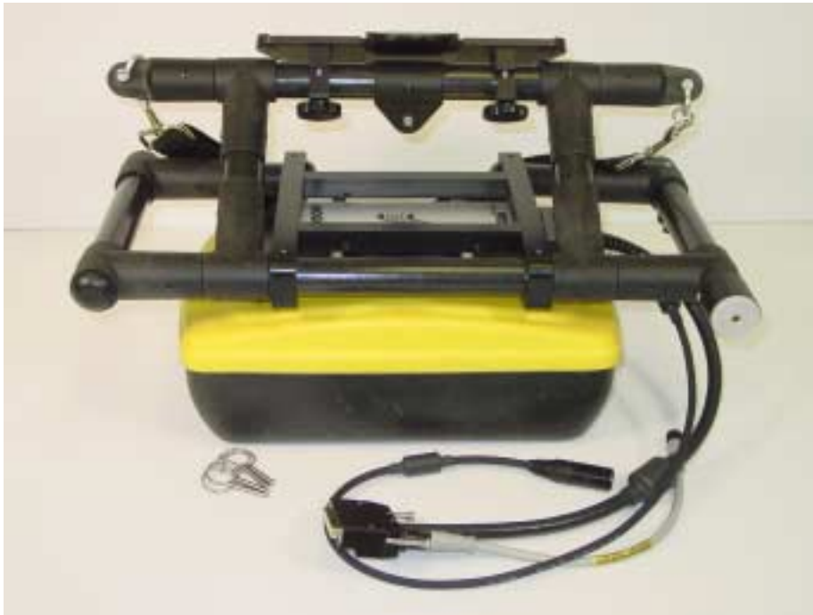
Figure: 7-10 Attach the end of the cable with the 37 pin (male) connection to the Noggin. Use a slotted screwdriver to tighten the connection.
