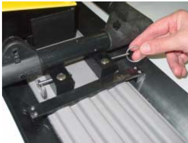
Figure: 4-12 Secure the SmartCart Separation Bars to the Noggin 100 by inserting the pins into each of the 8 post blocks.
