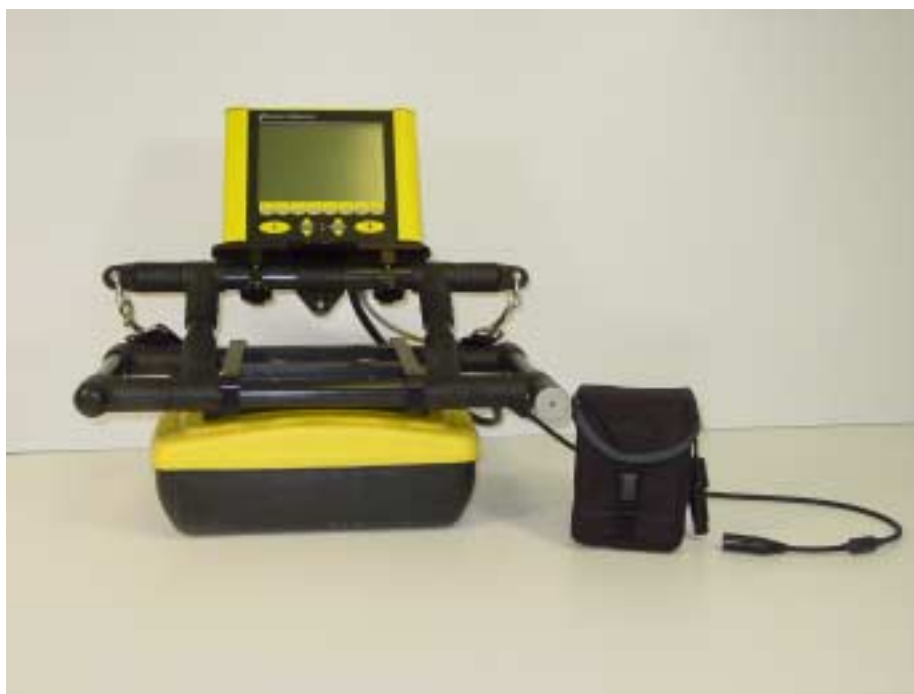
Figure: 7-14 The last connection on the cable is a cylindrical, 4 pin connector for the battery.
