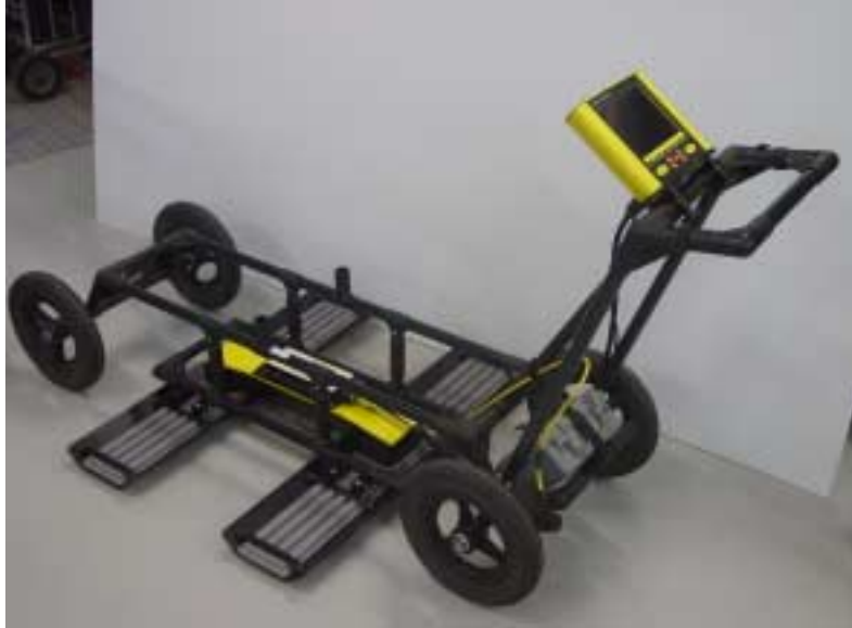
Figure: 4-11 Place the SmartCart over the Noggin 100 system with the 8 antenna mounting posts inserted in the post blocks. The 37 socket receptacle
