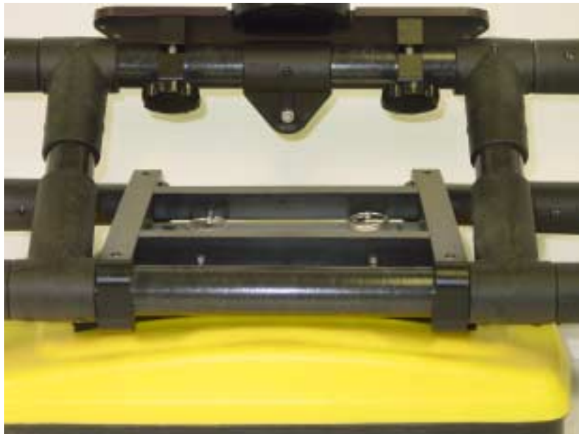
Figure: 7-9 Secure the frame to the Noggin by pushing the 4 clevis pins into the holes on the frame as shown.
