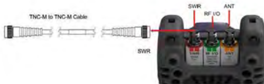
Figure 18: VSWR Calibration Setup Diagram
