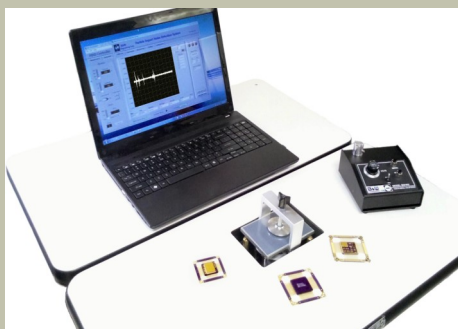
PC Controlled PIND Tester on test bench
