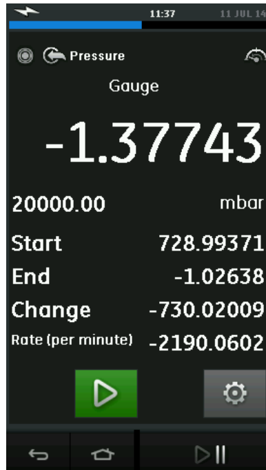
Figure 2-27 Leak Test Example
