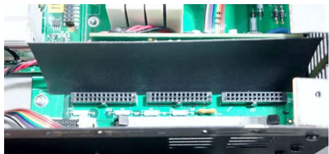
Figure 5.9 – Connectors location for front-end board replacement
