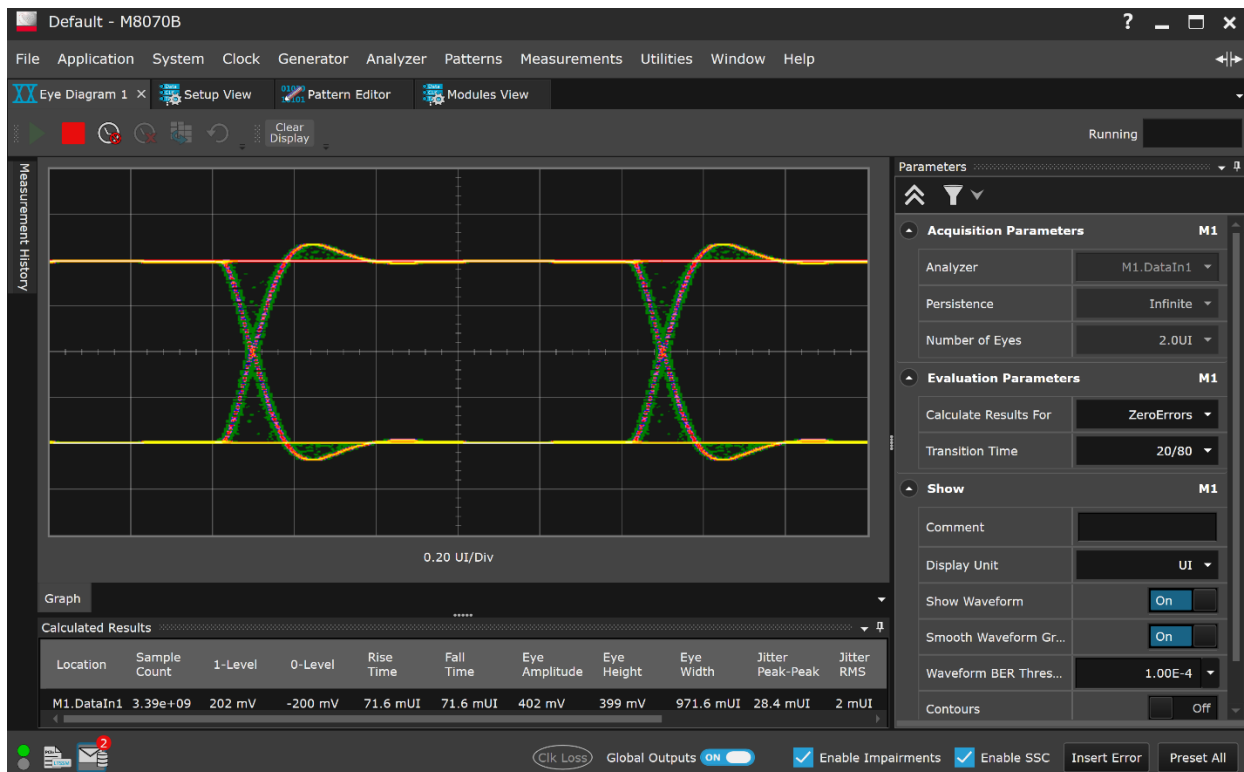
Figure 12. Eye diagram measurement with J-BERT M8020A Analyzer
