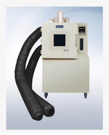
When ordering an RC, it is essential to specify a "local/remote" temperature sensor. This ensures accurate temperature measurement, accounting for blower-induced temperature rise and heat picked up in hoses.
