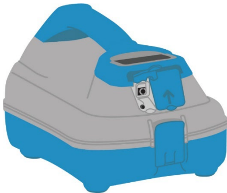
Figure 9.7: Transmitter DC Input
