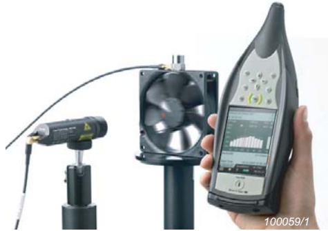
Fig. 10 Vibration measurement using a hand-held analyzer and Laser Tacho Probe Type 2981
