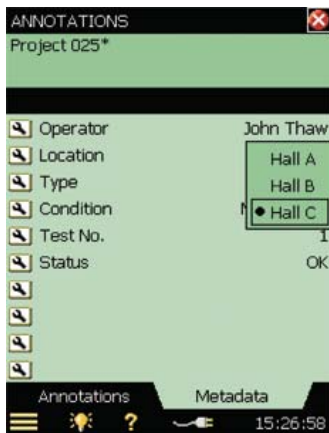
Fig. 11 The Annotations page showing six user- defined metadata items and a pick-list for the Location entry
