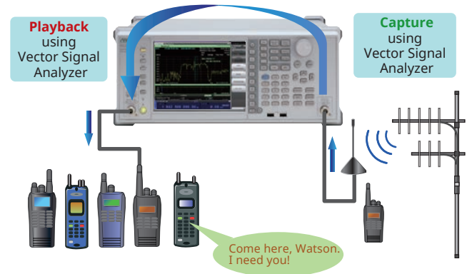
Repeatably Test Device Performance using “Real-World” RF Environments
