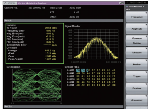
4FSK Modulation Analysis Measurement Example
