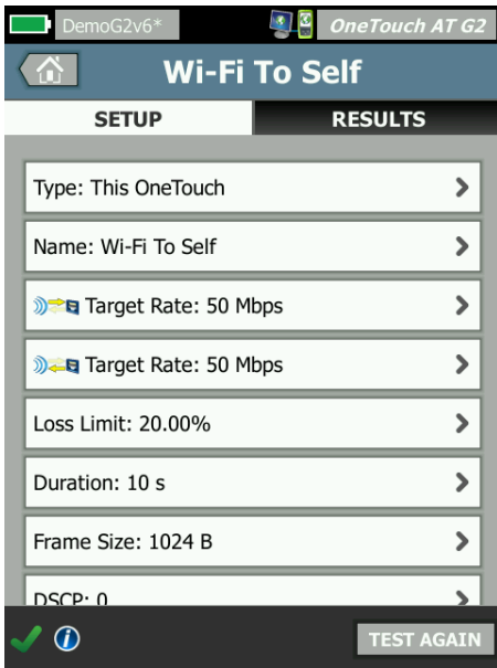
Figure 11: Simple setup to verify Wi-Fi or Wired Ethernet throughput against an endpoint on the wired network.
