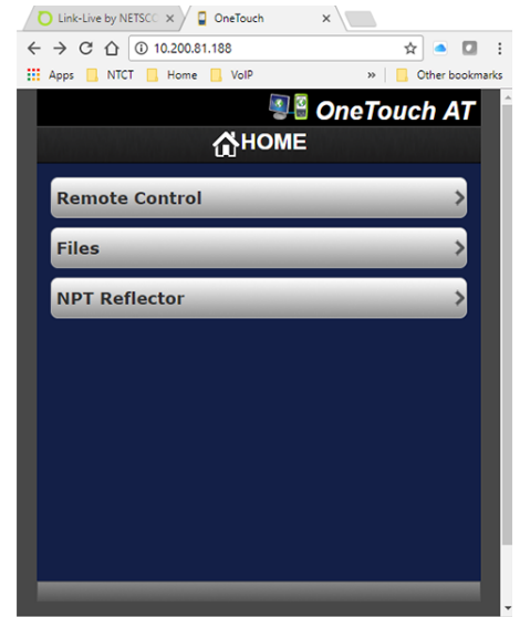
Figure 13: OneTouch web server for remote file retrieval and/or download the NPT Reflector software.
