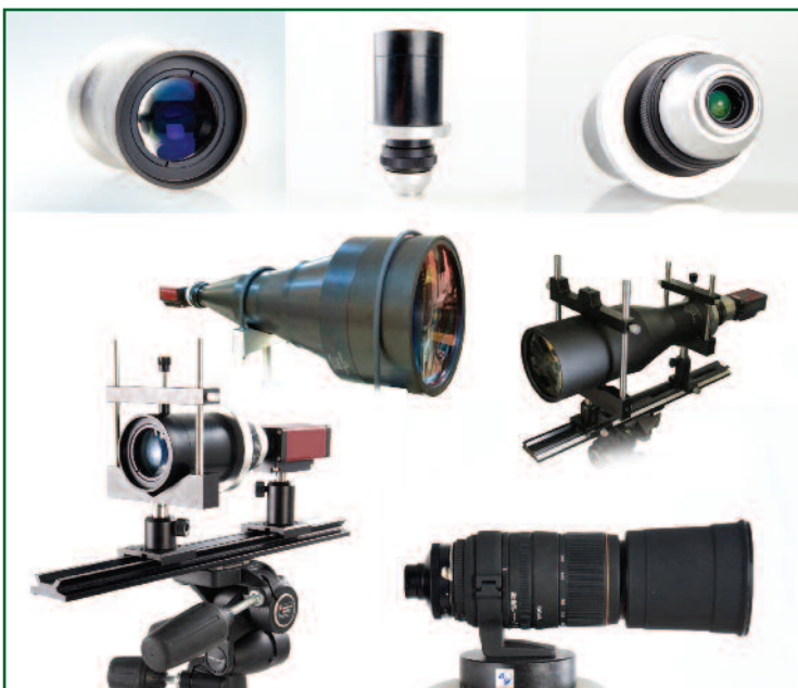
Figure 5. Selection of materials testing lenses, some shown with different translation stages that support the camera and lens and allow movement for focusing.
