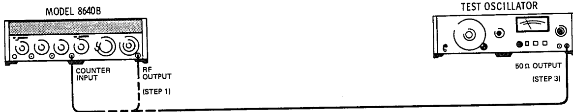
Figure 4-28. Counter External Sensitivity Test Setup
