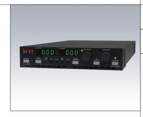
The cooling air intake is at the front and sides with exhaust at the rear and sides. Variable speed fans are controlled as a function of ambient air temperature and load, thus reducing acoustic noise and increasing fan life. This allows supplies to be stacked one directly on top of another without space in between, yielding maximum rackmount packing density and a wide operating temperature of 0-50° C. An optional rackmount kit is available to easily mount one or two units side-by-side.
