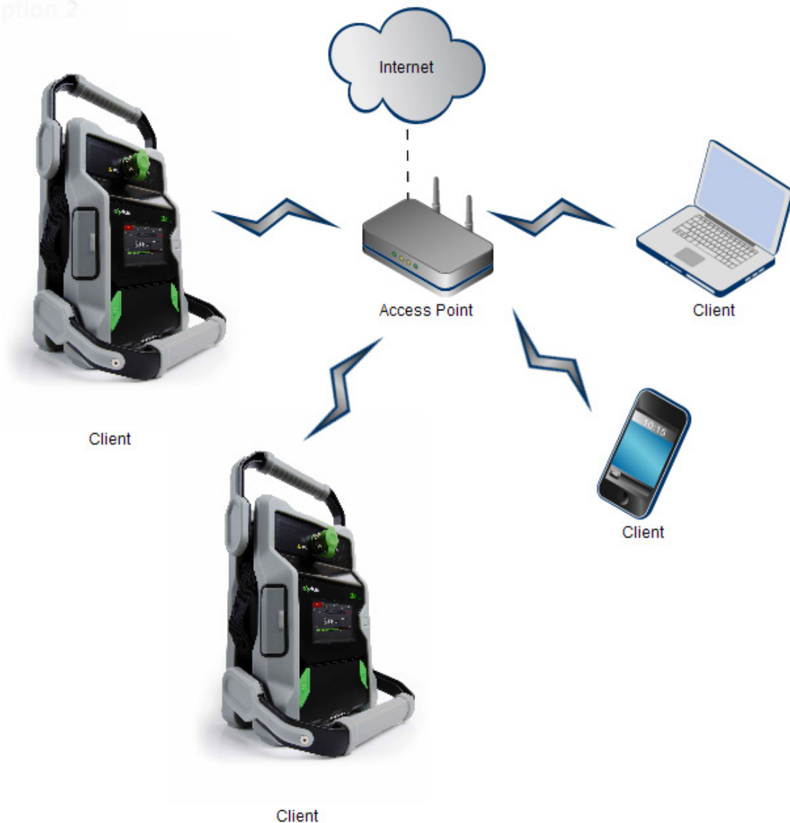
Figure 69 Wi-Fi Connection Options (external access point)
